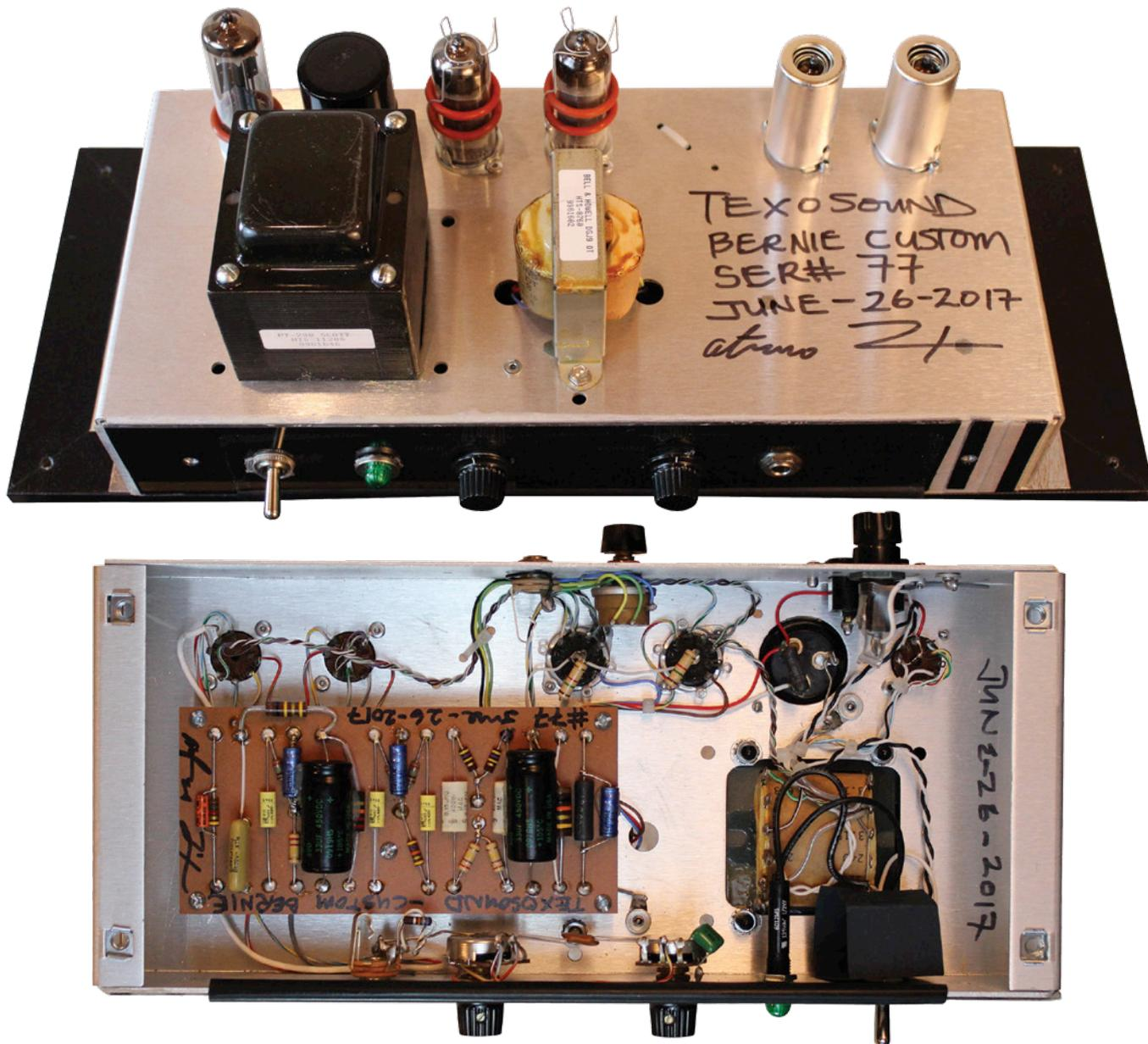
my Texosound EF86,” he adds. Tube-wise, the EL84s are a pair of respected NOS Russian military stock from the Reflektor plant, and the ECC83s in this example are from Mullard and RCA.
